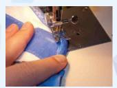
14. Stop sewing with a machine knot approximately 2 inches from where you started. Sew the loose ends of the FOE right sides together. Make sure it will cover the remaining distance without bunching or too much stretching and trim excess close to stitching. Finishing sewing FOE to diaper.
